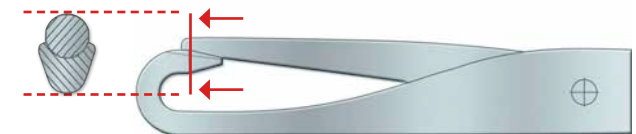
Prim latch type needle (latch without groove)
