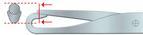
Needles with grooved hook: spoonless latch
